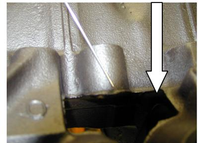
**2. Temporarily position the rear aluminum brace in place and observe how much metal may need to be ground away from the cast iron center lifter brace in order to permit passage of the clamping bolt. You MAY have to grind a small amount of material from the center of the block (see photo 2) for the MEGA BRACE clamping bolt.**
