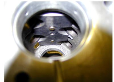
**5. Carefully and thoroughly clean the outside surfaces of the lifter bores as well as the notches in the aluminum lifter braces with brake parts cleaner, or, a similar product that can remove grease without leaving an oily residue.**
