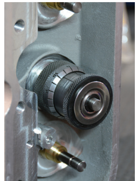
The titanium valves were installed in the RHS heads so the spring height could be double-checked. The trick tool steel retainers were loaded into the height checker, and all measurements were recorded.
