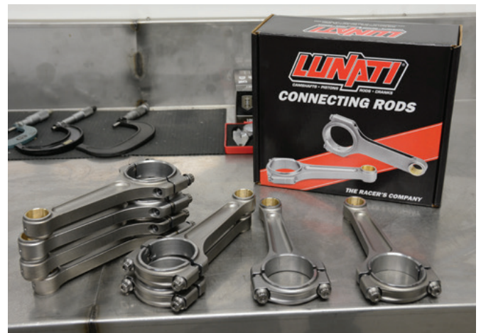
Lunati Rods were checked and balanced before hand.
