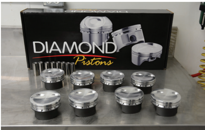
The pistons from Diamond were works of art. They were coated on the bottom and featured beautiful CNC work on the crown — no extra work needed.
