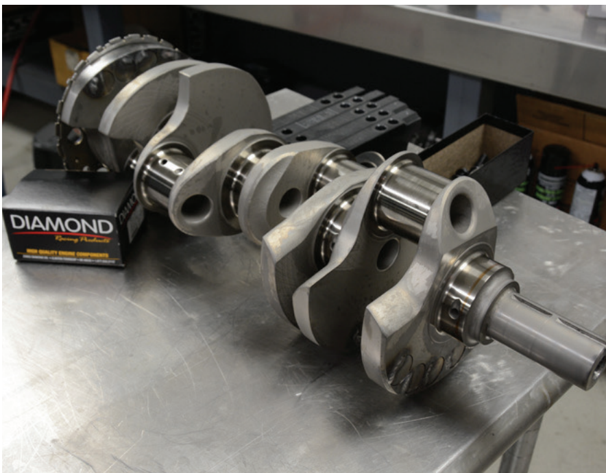
The Lunati crankshaft was balanced in-house.
