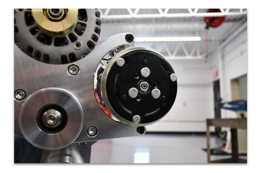
From the rear, attach the ac compressor to the back bracket using an 8mm bolt and washer/ nut.
