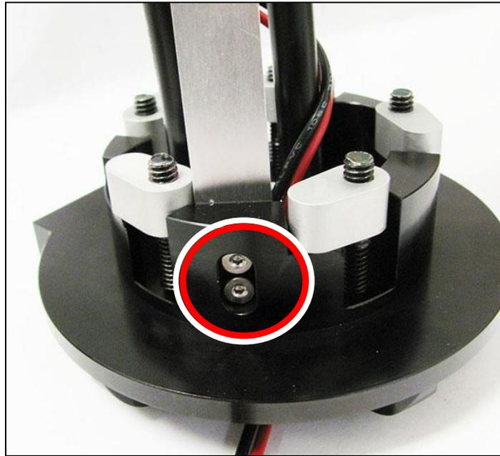
**11. Installing pump for 12-129, 12-130, 12-132, 12-134, 12-136, 12-137, 12-158, & 12-159 Universal Pump Hanger Assy (Billet Return & Cast Return/Returnless)**
