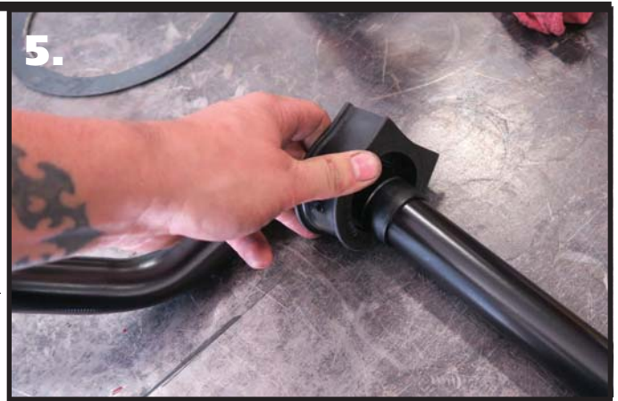
5. Open the SwayBar Bushing at the split and slide it OVER the Delrin Liner. Do this on both Delrin Liners.
