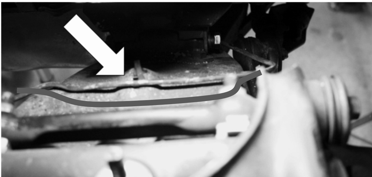
Picture #2, Brake Line, relocate from Arrow to Gray Line Area
