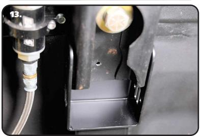
**13. Image 13** shows the 1/4" hole drilled in the OEM subframe. This hole will now get drilled to 1/2" diameter.
