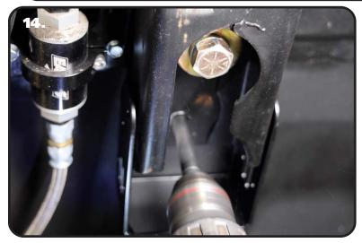
**14.** Use a 1/2" drill bit to drill out the 1/4" hole.
