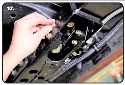
**17.** Install a 5/16" flat washer on each of (4) 5/16"-18 x 1" bolts. Insert a bolt/washer in each of the 4 holes. Install a 5/16" flat washer and 5/16"-18 nylok nut on the threads of each of the (4) bolts. Torque the hardware to 25 ftlbs.
