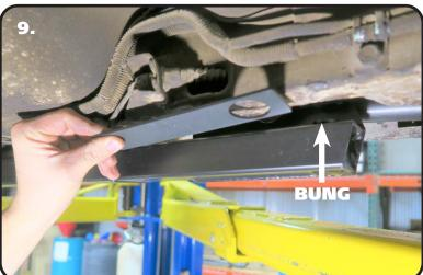
**9.** Place the shim on top of the subframe connector tube with the hole in the shim over the rear bung.
