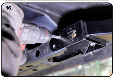
**16.** The 4 side frame mounting holes in the front of the subframe connector will be used as a template to drill the new holes in the OEM subframe. Drill the 4 holes with a 5/16" drill bit.
