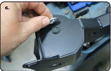
6. The leaf spring mounting holes in the subframe connector's are 5/8" for many aftermarket suspensions. The kit includes T-bushings for using 1/2" hardware. If you are using 1/2" hardware, insert a t-bushing in each leaf spring mounting hole. The large OD will be on the outside of the leaf spring pocket.
