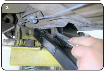
**7.** Attach the rear of the subframe connector to the front of the leaf spring. Install the leaf spring bolt from the outside of the car with the nut to the inside. The leaf spring bolt will need to be tightened before the subframe connector is installed.
