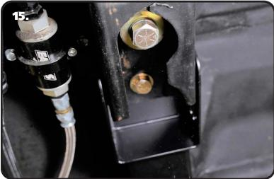
**15.** Install a 1/2" flat washer on a 1/2"-13 x 1 1/4" hex bolt. Insert the bolt in the drilled 1/2" hole. Install a 1/2" flat washer and 1/2"-13 nylok nut on the threads of the bolt. Torque the hardware to 75 ft-lbs.
