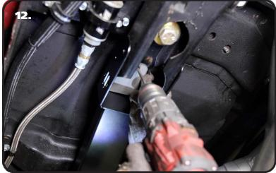
**12.** Hold the template in place and use it as a guide to drill a 1/4" hole in the OEM subframe.
