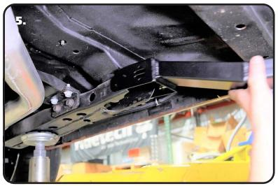
**5.** The kit includes a Driver and Passenger subframe connector. The leaf spring mount is positioned to the outside of the car with the subframe connector tube dipping down to clear the floor pan. Insert the front of the subframe connecter so that the front ledge is sitting on TOP of the OEM subframe.
