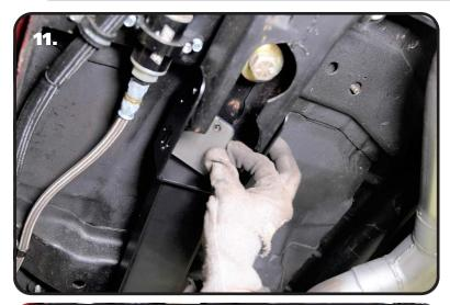
**11.** Insert the drilling template in the opening at the connection area of the connector/subframe. The temple has a small hole the is use as a guide to drill a 1/4" hole in the top of the OEM subframe. The template will nest against the front edge of the subframe connector. The narrow side of the template will point forward.
