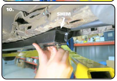
**10.** Install a 3/8" split lock washer and 3/8" flat washer on a 3/8"-16 x 3" hex bolt. Insert the bolt/washer in the inner hole of the subframe connector. This hole goes through the tube of the subframe connector and lines up with the u-nut that is in the OEM frame rail. Thread the bolt into the u-nut. Leave the hardware loose until later. Tighten the (3) REAR subframe mounting bolts that to 30 ftlbs.
