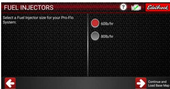
8. The Wizard will automatically start loading a base map. When the map is finished loading, you will be prompted to power cycle the ECU. Turn the ignition switch off, wait for the main relay to click off (approx. 10 seconds) and then turn the ignition switch back on. Tap OK to close the popup window then tap the Right Arrow to continue.
