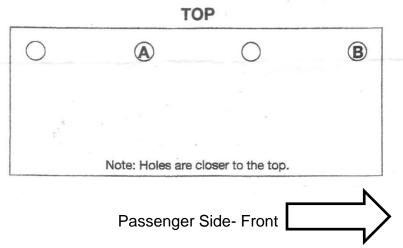
Note: It has been brought to our attention that some late 70's Pontiac blocks have a boss that interferes with the adaptor plate. If this is the case, the boss will have to be ground for clearance or drilled or tapped to 7/16" to bolt the mount directly to the block. If drilled or tapped, this side will not require an adaptor plate. **Adaptor plates must fit flat.**
