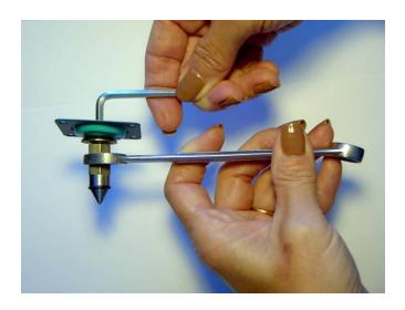
Step 7: Insert the diaphragm assembly and attached bypass plunger into the top of the housing:
