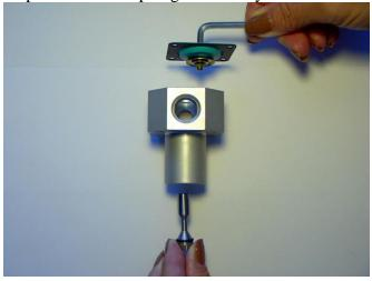
Step 6: Screw the bypass plunger onto the diaphragm assembly and tighten (make sure the sealing washer stays in place):
