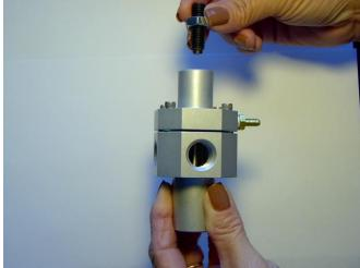
Step 2: Using an allen wrench, remove the four screws holding the cap to the housing:
