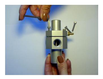
Install the pressure adjustment set screw and jam nut:
