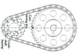
carefully inspect the crankshaft sprocket equivalent Note the position of mark on the outside the position of the each keyway on the gear tooth. inside diameter Before assembl timing and
