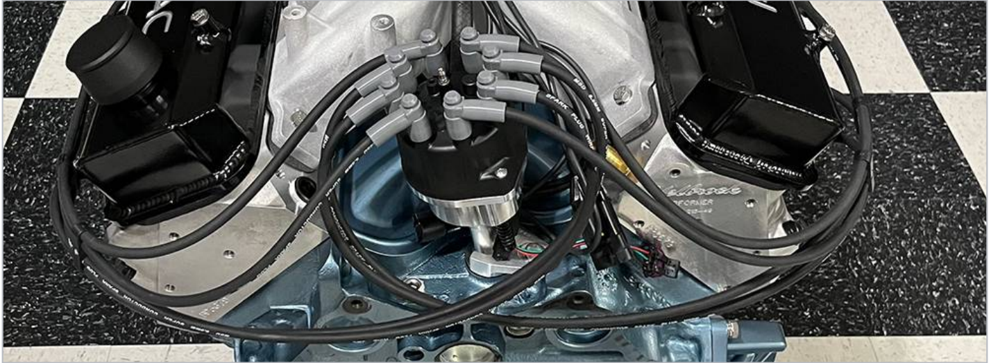
Finished Butler routing — MSD Black 8.5mm Super Conductor on a Pontiac V8.
